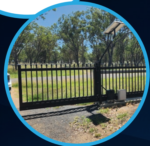
Cantilever design – no track across driveway
